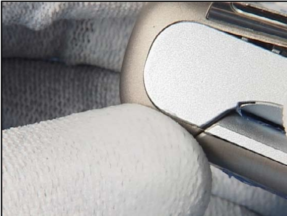
19. Click the snaps into their places, beginning from the upper side of the ANTENNA CAP.
