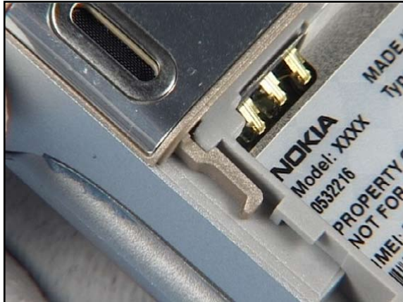
20. Note the correct positioning of the snaps before going on.
