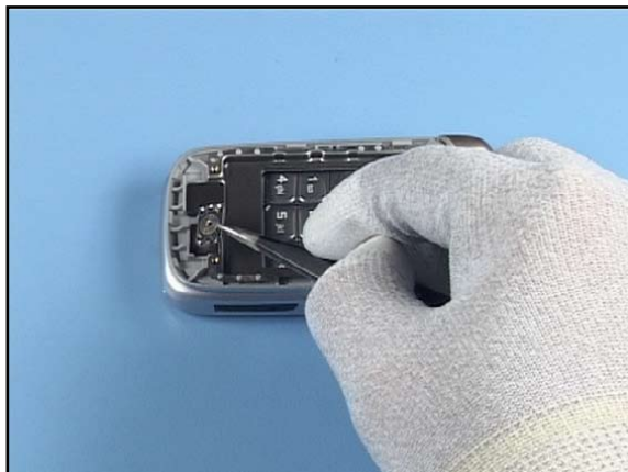
24. Insert the EARPIECE into ist recess. Note that a new speaker gasket must be fitted first.
