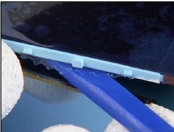
21. Release the LCD BACK ADHESIVE with the SS-93.
