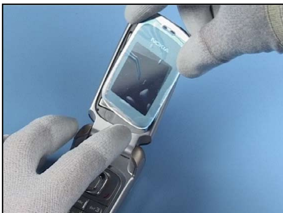
42. Fit the new LCD WINDOW, beginning at the hinge side.
