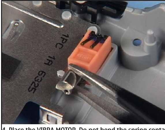
4. Place the VIBRA MOTOR. Do not bend the spring contacts.
