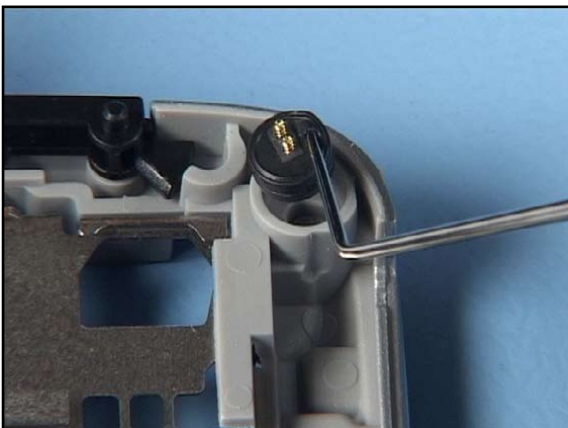
15. Ease the MICROPHONE with the dental pick.
