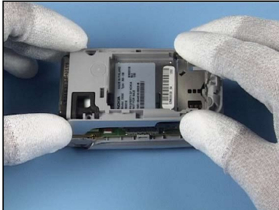
14. Now align the C-COVER above the A-COVER and push it down evenly.
