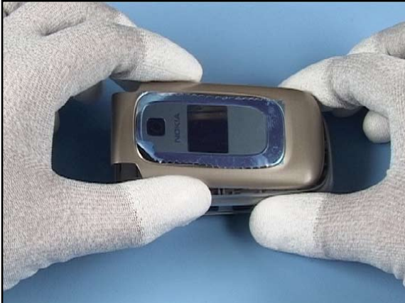
7. Shift the B-Cover Assy to the hinge direction and lift it up.
