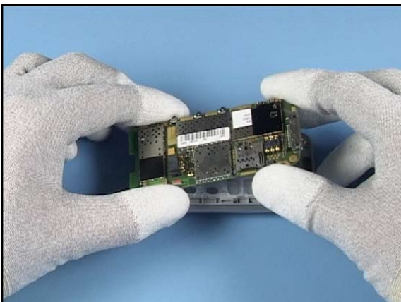
11. Lift up the ENGINE MODULE, keep in mind that the flex foil is still connected.
