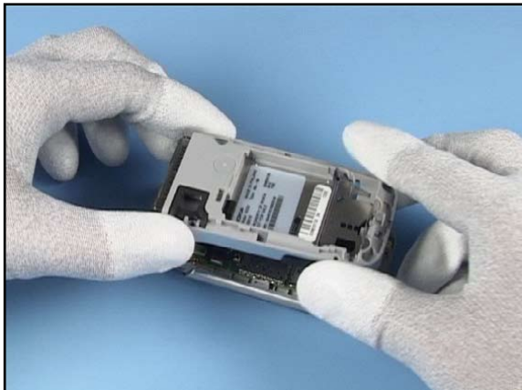
10. Carefully lift up the cover.
